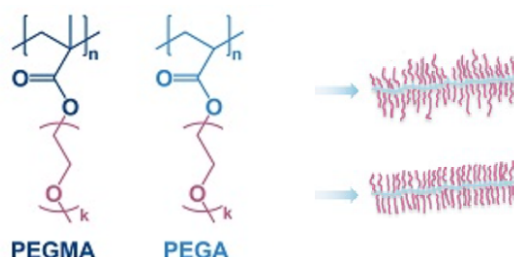
Figure 1: On the left the molecular structures of PEGMA and PEGA. k can be variable (dispersed side chains) or constant (discrete side chains). On the right a representation of the final graft polymer brushes with either dispersed (top) or discrete (bottom) side chains
