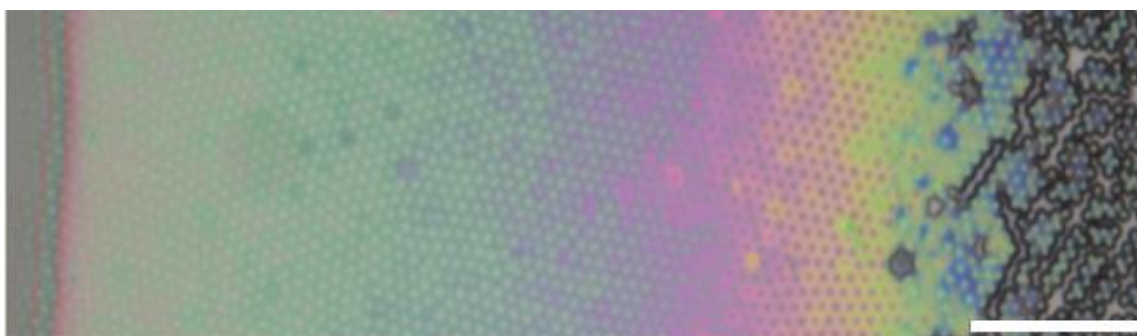
Figure 1: Microgel monolayer during different states of drying (from right to left) on a hydrophobic substrate. Scale bar = 10 \mu\text{m} .
