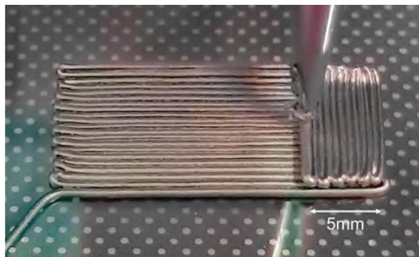
Figure 1: *DIW of PANI, fabricating a rectangular grid structure for EM shielding*
