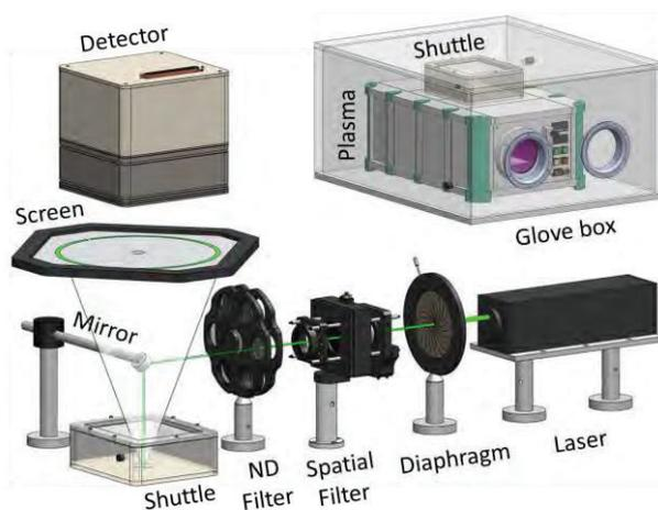
Figure 1: Schematic of plasma exposure and small-angle light scattering (SALS) setup in controlled environment to study the environmental effects on spontaneous wrinkle formation in plasma oxidised PDMS.
