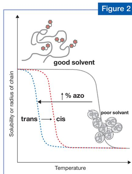
**Figure 2:** Principle of light-triggered collapse and/or aggregation of polymer chains. Increasing the density of (hydrophobic) photochrome in chains shifts LCST to low T; polarity recovery upon exposure to UV light increases LCST.
