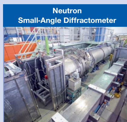
Figure 3: Photo of the JCNS SANS instruments KWS1 and 2 at FRM II in Garching (Germany).
