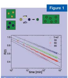
Fig. 1: Schematics of the isotopic substitution SANS experiment to observe the equilibrium exchange kinetics in micellar solution (top) and its result, the logarithmic decay of the excess of labelled chains (bottom).
